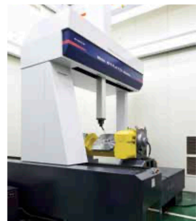
Accuracy measurement with large 3 Dimensional Measuring Machine
