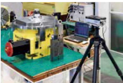
Indexing Accuracy Measurement by Laser
